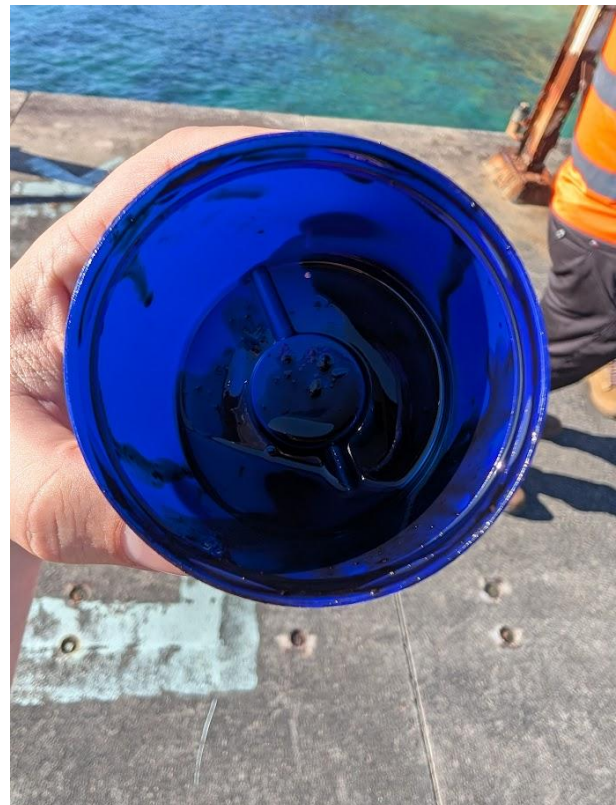
Photo 10 Substance Extracted from CHS Piles
