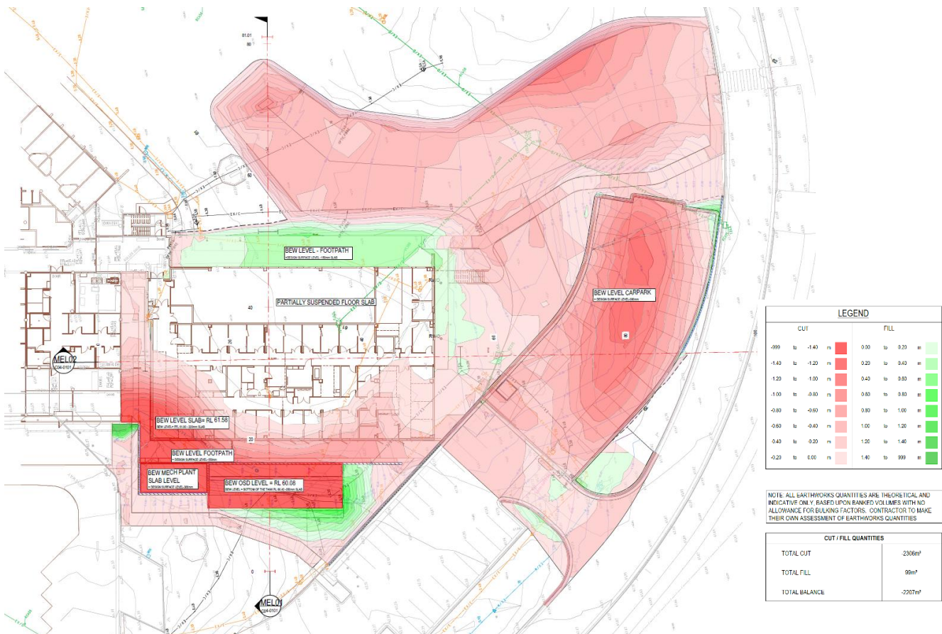
Figure 39 – Bulk earthworks and cut/fill drawing (ACOR)
