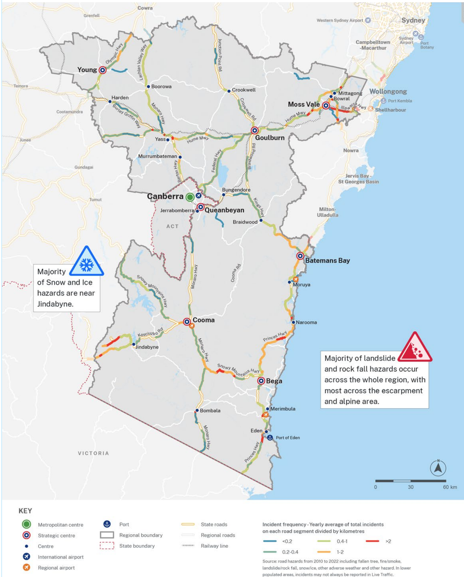
Figure 18. Environmental hazards on the South East and Tablelands region road network between 2012 and 2022
